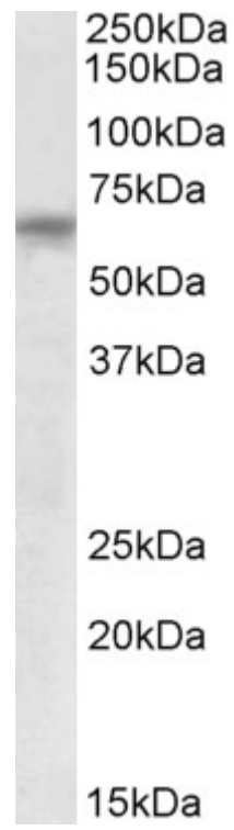
EB09988 (0.2µg/ml) staining of Human Testis lysate (35µg protein in RIPA buffer). Primary incubation was 1 hour. Detected by chemiluminescence.
