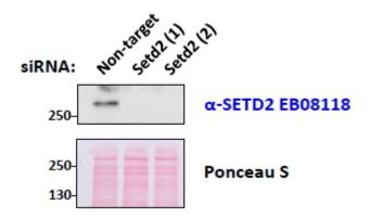
EB08118 (0.5µg/ml) staining of mouse fibroblast lysates transiently expressing different siRNA in second and third lane (35µg protein in RIPA buffer). Primary incubation was 1 hour. Detected by chemiluminescence.
